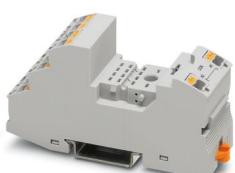
Relay base RIF-2..., for industrial relay with 2 or 4 changeover contacts, Push-in connection, plug-in option for input/interference suppression modules, for mounting on NS 35/7,5
