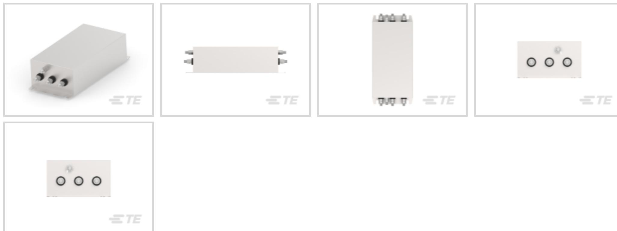
Current Rating: **150 A**Input Termination Type: **Threaded Bolt**Output Termination Type: **Threaded Bolt**Wiring Configuration: **DELTA (3 wire + ground)**Operating Voltage: **520 VAC**
