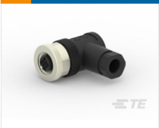
TE Part # T4112001051-000 M12,FEMALE,RA,A CODE,5P,PG7, GOLD
