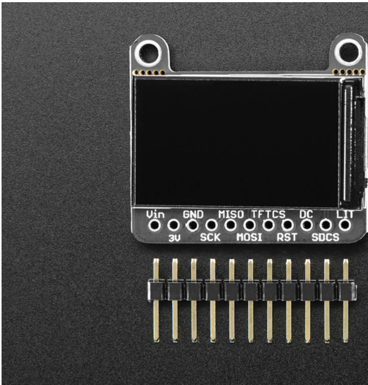
Our breakout has the TFT display soldered on (it uses a delicate flex-circuit connector) as well as a ultra-low-dropout 3.3V regulator and a 3/5V level shifter so you can use it with 3.3V or 5V power and logic. We also had a little space so we placed a microSD card holder so you can easily load full color bitmaps from a FAT16/FAT32 formatted microSD card. The microSD card is not included, [but you can pick one up here](http://adafru.it/102) (<http://adafru.it/102>).
