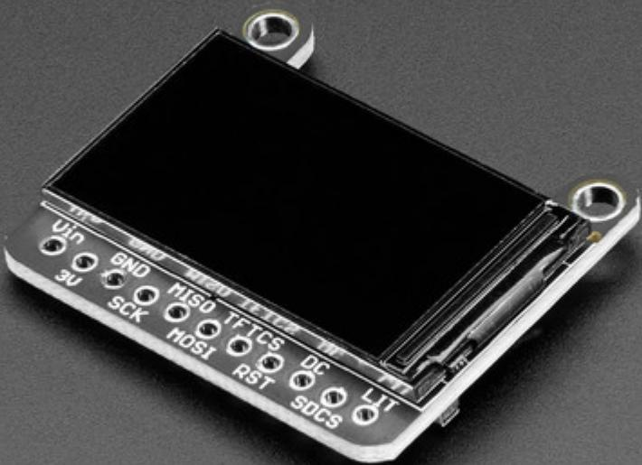
Say hello to our **1.14" 240x135 Color TFT Display w/ MicroSD Card Breakout** - we think it's **T-F-Terrific!** It's the size of your thumbnail, with glorious 240x135 high res pixel color. This very very small display is only 1.14" diagonal, packed with RGB pixels, for making very small, high-density displays.
