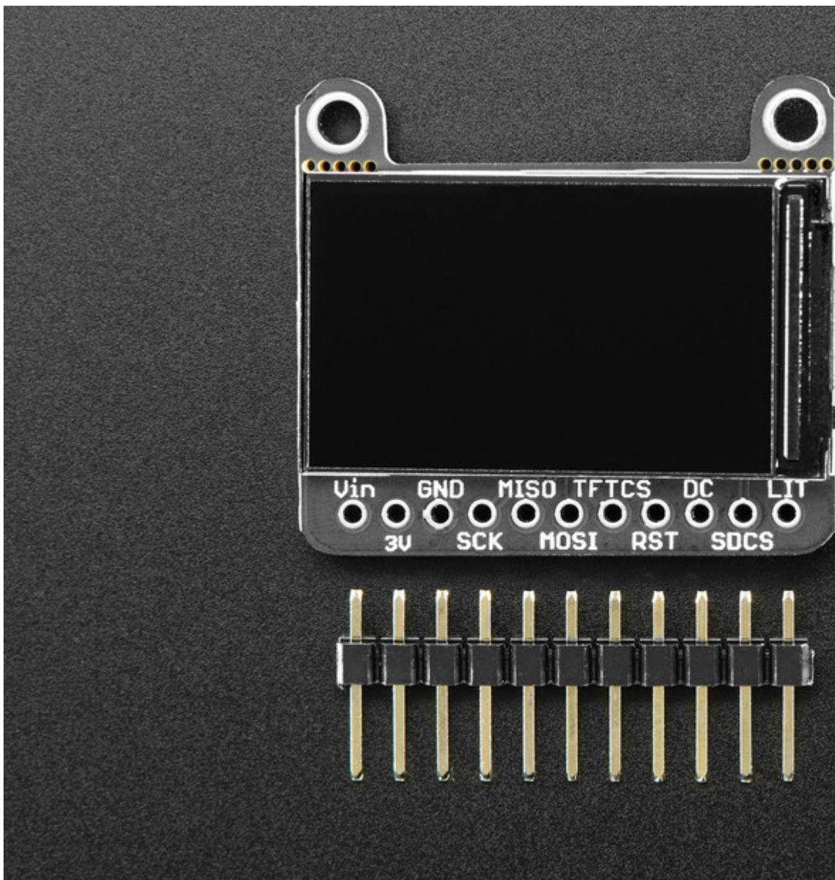
This color display uses SPI to receive image data. That means you need at least 4 pins - clock, data in, TFT cs and d/c. If you'd like to have SD card usage too, add another 2 pins - data out and card cs. However, there's a couple other pins you may want to use, lets go thru them all!
