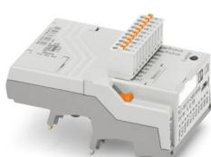
PLC logic basic module with RS-485 connection for Modbus/RTU communication, with 16 I/Os, for plug-in connection to 8 digital or analog PLC-INTERFACE terminal blocks, can be extended to 48 I/Os, real-time clock, micro USB female connector, accommodates memory module and Bluetooth adapter, Push-in connection
