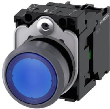
Illuminated pushbutton, 22 mm, round, plastic with metal front ring, blue, pushbutton, flat, momentary contact type, with holder, 1NO, LED module with integrated LED 230 V AC, screw terminal, with laser labeling, upper case and lower case, always upper case at beginning of line
