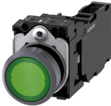
Illuminated pushbutton, 22 mm, round, plastic with metal front ring, green, pushbutton, flat, momentary contact type, with holder, 1 NO+1 NC, LED module with integrated LED 230 V AC, screw terminal, with laser labeling, inscription or symbol Customer-specific selection with SIRIUS ACT configurator (CIN)
