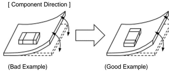
Locate chip horizontal to the direction in which stress acts.
