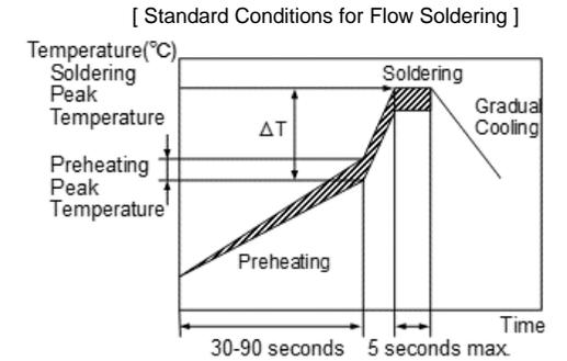
[ Allowable Flow Soldering Temperature and Time ]
