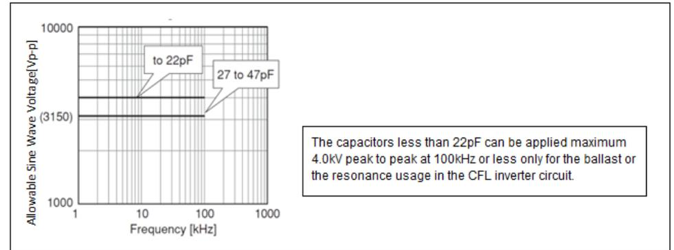
The capacitors less than 22pF can be applied maximum 4.0kV peak to peak at 100kHz or less only for the ballast or the resonance usage in the CFL inverter circuit.
