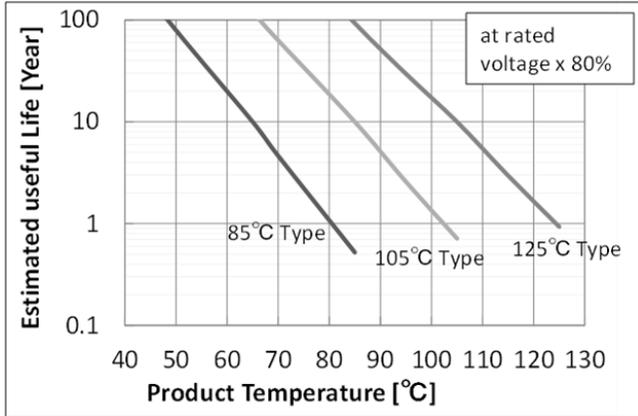
Murata's General MLCC products are designed for use in devices with a typical lifetime around 10 years. Murata's general MLCC products are designed so that the estimated useful life can be extended longer than 10 years under the following conditions: 「80% of the rated voltage or less, Maximum operating temperature -20 degree C or less」 The estimated useful life under actual operating conditions can be approximated from the chart.
