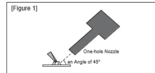
3. Optimum solder amount when re-working with a soldering iron
