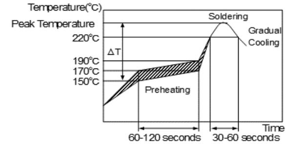
[ Allowable Reflow Soldering Temperature and Time ]
