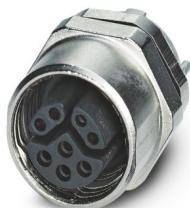
Device connector rear mounting, Ethernet CAT5 (IEC 11801:2002), 8-position, Socket, straight, M12-SPEEDCON, coding: Y, PCB mounting, M12 x 1, THR solder connection, Alternative product in accordance with RoHS II without Exemption 6c (Pb < 0.1 %) item no.: 1239824
