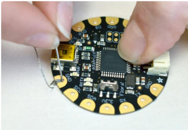
Stitch a few times around the GND pad and end on the back side of the fabric. Tie the tail and the working thread into a square knot, tight against the fabric.
