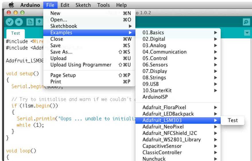
Open the special Adafruit version of the Arduino IDE and navigate to File-->Examples-->Adafruit\_LSM303-->Test to open the accelerometer test sketch. For more information on programming the Flora, check out the [Getting Started with FLORA \(https://adafru.it/aSZ\)](https://adafru.it/aSZ) guide.
