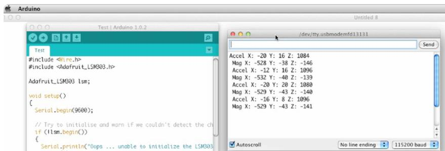
Open the serial monitor and watch the accelerometer values pour in!
