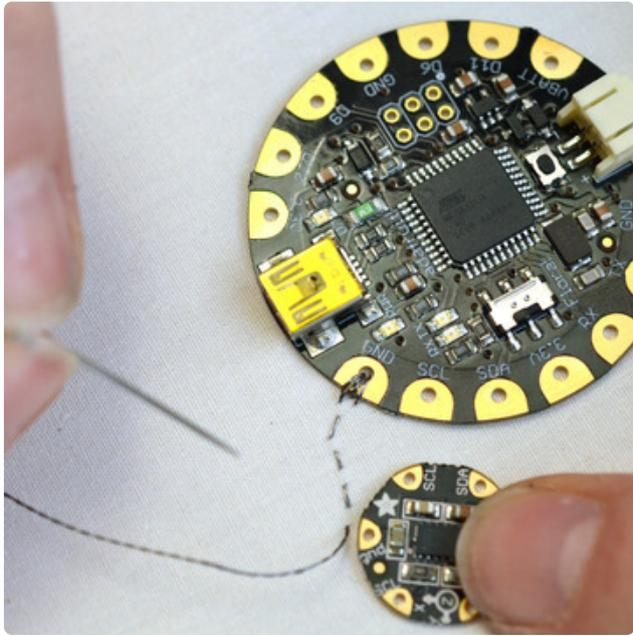
Stitch a path over to the gnd pad on the Flora accelerometer. When you get there, stitch a few times around the sensor's gnd pad.
