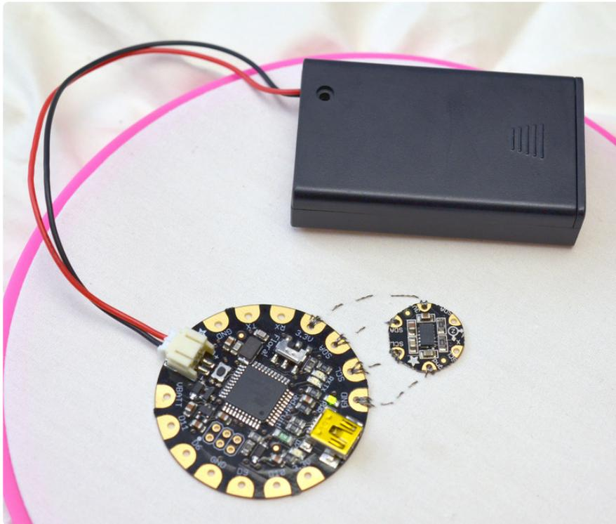
Modify this sample sketch to integrate this sensor into your project. Debugging over USB is helpful to see the ranges of numbers your sensor provides, but once your code is solid, you can disconnect from the computer and power your project with a 3xAAA battery holder.
