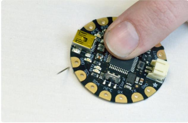
Bring your needle through the back of the fabric to the front next to the GND pad on your Flora. Leave the last few inches as a tail on the back side of the fabric.
