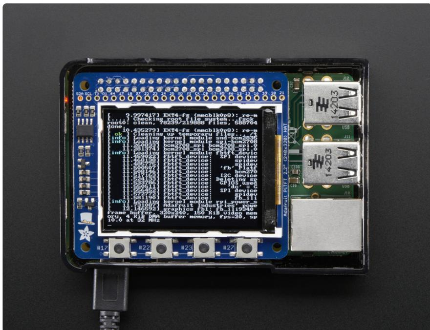
To make it super easy for use: we've created a custom kernel package based off Notro's awesome framebuffer work, so you can install it over your existing Raspbian (or derivative) images in just a few commands.
