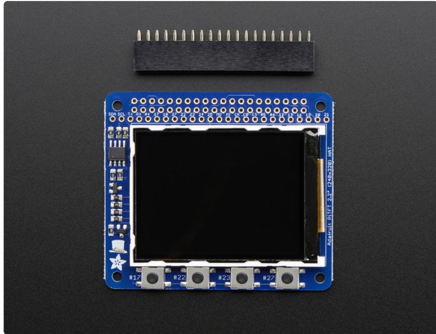
Comes as a fully assembled display PCB and an additional 2x20 GPIO header. Some light soldering is required to attach the 2x20 GPIO header to the HAT but it's fast and easy for anyone with a soldering iron and solder
