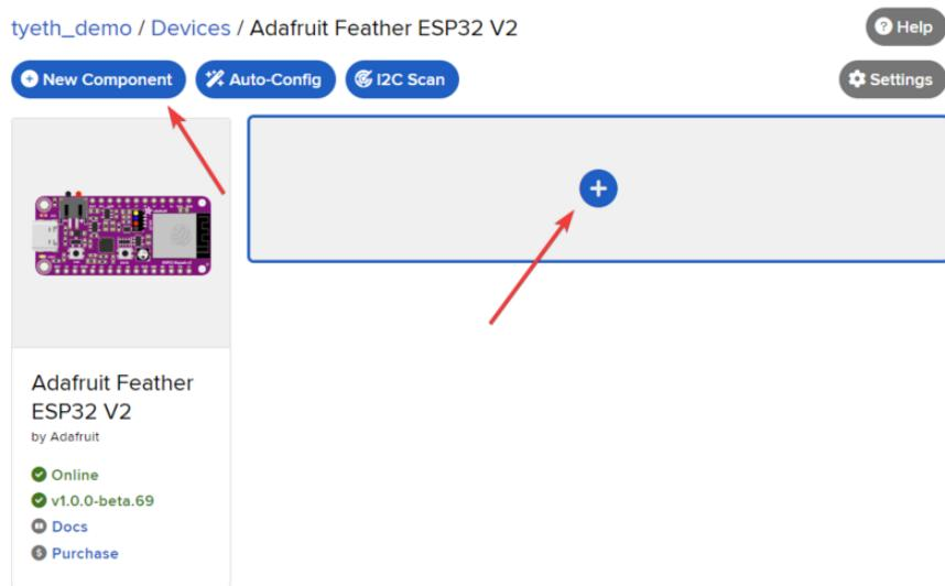
Adafruit IO supports a large amount of components. To quickly find your sensor, type **SHT3** into the search bar, then select the matching **SHT30/SHT3x** component.
