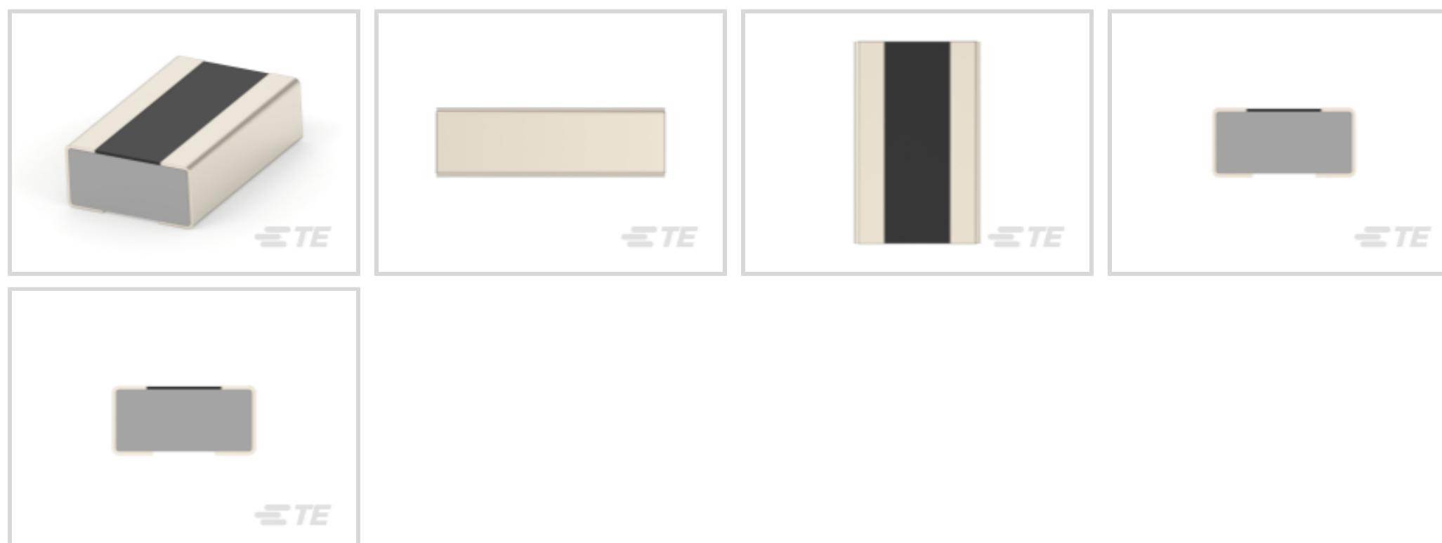
Resistor Type: **Current Sensing Resistor**Element Type: **Thick Film**Package Size Code: **0508**Power Rating: **1 W**Resistance Value: **.082  $\Omega$**
