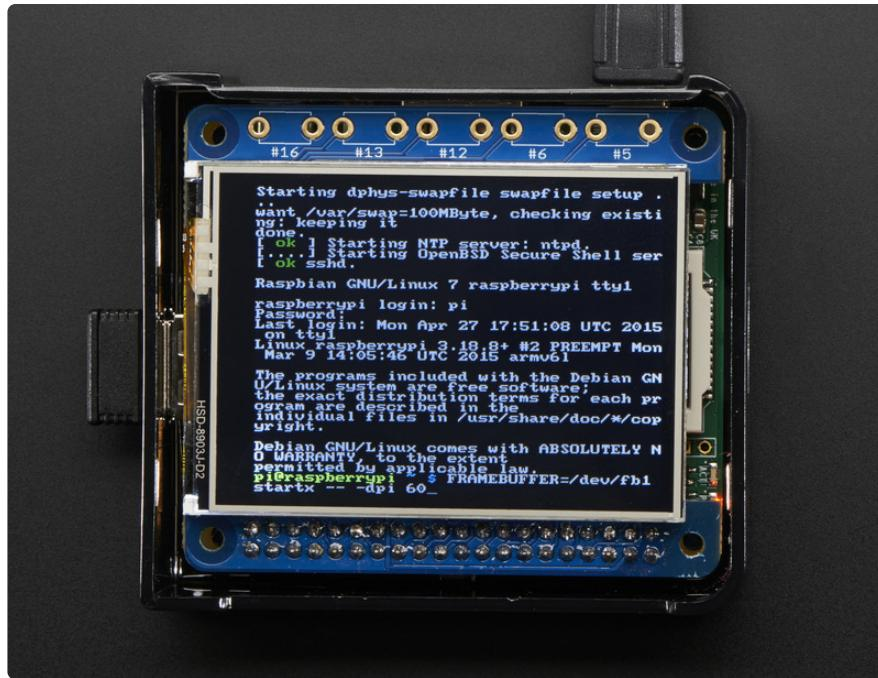
To make it super easy for use: we've created a custom kernel package based off of Notro's awesome framebuffer work, so you can install it over your existing Raspbian (or derivative) images in just a few commands.
