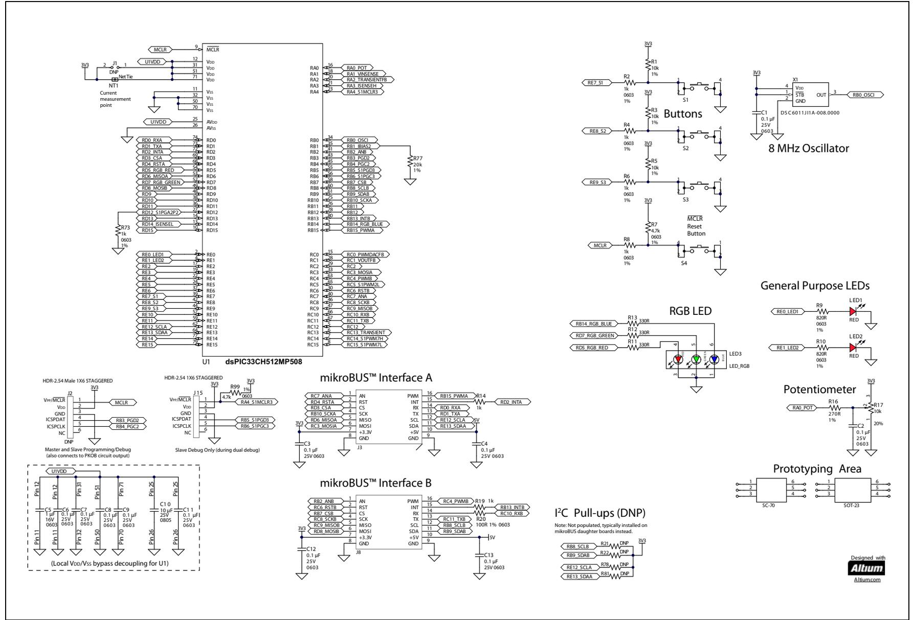
**FIGURE A-2: dsPIC33CH CURIOSITY BOARD LAYOUT SCHEMATIC REV. 1.0 (SHEET TWO OF FOUR)**
