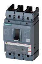
circuit breaker 3VA5 UL frame 250 breaking capacity class H 65kA @ 480V 2-pole, line protection TM230, FTAM, In=90A overload protection Ir=90A fixed short-circuit protection Ii=5...10 x In without connection
