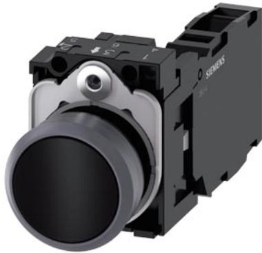
Pushbutton, 22 mm, round, plastic with metal front ring, black, pushbutton, flat, momentary contact type, with holder, 1 NO+1 NC, screw terminal, with laser labeling, inscription or symbol Customer-specific selection with SIRIUS ACT configurator (CIN)
