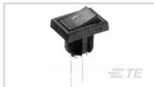
Switch Type: **Power**Indicator/Imprint Legend: **None**Panel Cutout Size: **11.3 x 12.06 mm [ .445 x .475 in ]**Switch Contact Plating Material: **Silver**Configuration (Pole-Throw): **Single Pole - Double Throw**
