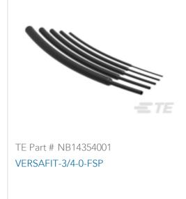
Black, 2:1, Single Wall Tubing, Shrinks To .125 in [3.17 mm], Irradiated Modified Polyolefin, .28 in [7.11 mm] Inner Diameter, RAYCHEM Versafit
