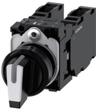
Selector switch, illuminable, 22 mm, round, plastic, white, selector switch, short, 3 switch positions I-O-II, latching, 10:30h/12h/13:30h, with holder, 2 x 1 NO+1 NC, screw terminal, with laser labeling, inscription or symbol Customer-specific selection with SIRIUS ACT configurator (CIN)
