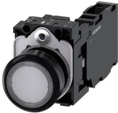
Pushbutton, 22 mm, round, plastic, clear, pushbutton, flat, momentary contact type, with holder 1 NO+1 NC, screw terminal, Z=20-unit packaging
