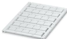
Marker for terminal blocks, Sheet, white, unlabeled, can be labeled with: TOPMARK NEO, TOPMARK LASER, BLUEMARK ID COLOR, BLUEMARK ID, BLUEMARK CLED, THERMOMARK PRIME, THERMOMARK CARD 2.0, THERMOMARK CARD, mounting type: snapped, for terminal block width: 12 mm, lettering field size: 10.8 x 9.6 mm, Number of individual labels: 30
