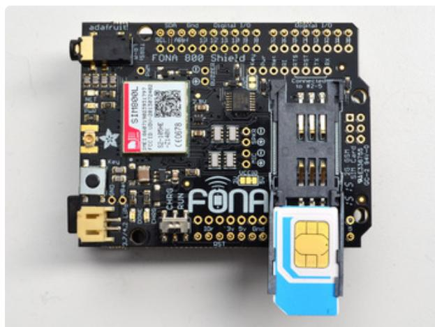
Insert the SIM with the gold pads facing up and the notch on the outer corner
