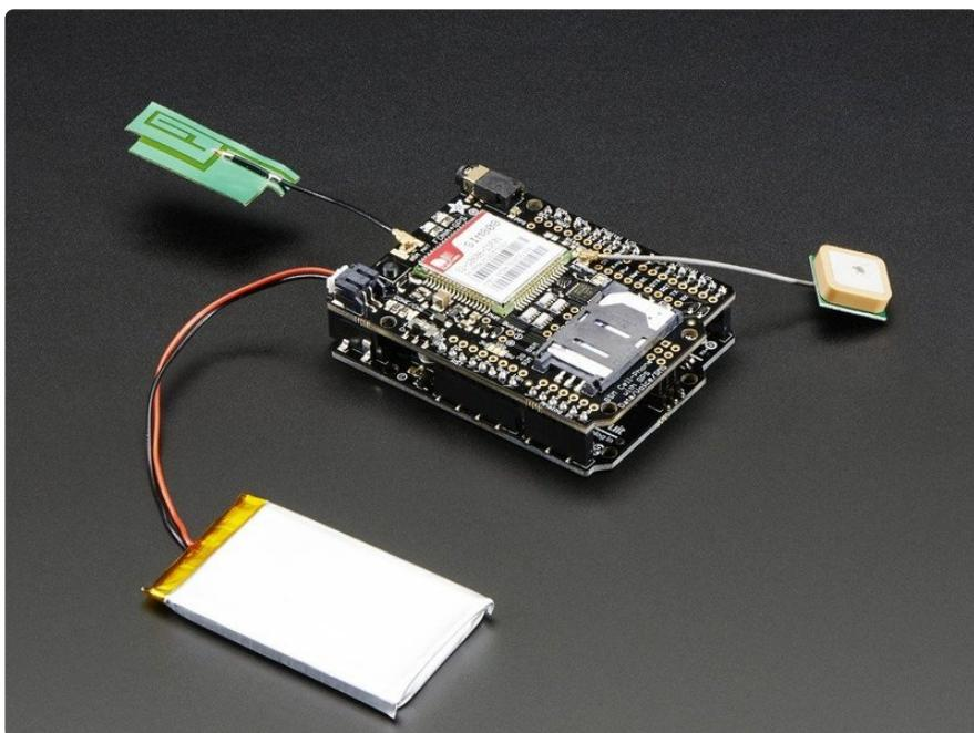
This shield fits right over your Arduino or compatible. At the heart is a powerful GSM cellular module (we use the latest SIM808) with integrated GPS. This module can do just about everything
