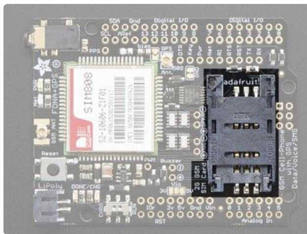
The SIM card holder is on the right side of the shield. It holds a very-standard "Mini SIM".
