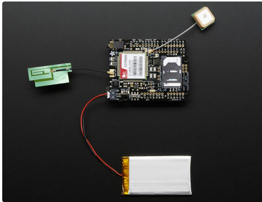
**Check polarity for the battery!**
