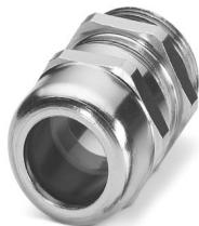
Cable gland, material for screw connection: Brass, nickel-plated, application: Standard, external cable diameter 10 mm ... 14 mm, shielding: no, connecting thread: M25 x 1.5, color: silver, with O-ring
