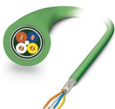
Data cable, PROFINET CAT5 (100 Mbps), 4-position, PVC/PVC, green RAL 6018, shielded, free cable end, on free cable end, cable length: Free entry (0.5 ... 400 m)
