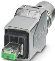
RJ45 connector, degree of protection: IP65/IP67, number of positions: 8, 1 Gbps, CAT5, material: Metal, connection method: IDC fast connection, connection cross section: AWG 23- 22, cable outlet: straight, Ethernet
