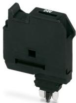
Fuse plug, Prior to replacing the cartridge fuse, disconnect the fuse connector from the basic terminal block., nom. voltage: 500 V, nominal current: 6.3 A, connection method: Plug-in connection, fuse type: G / 5 x 20, mounting type: Plug-in mounting, color: black
