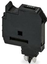
Fuse plug, Prior to replacing the cartridge fuse, disconnect the fuse connector from the basic terminal block., nom. voltage: 500 V, nominal current: 6.3 A, fuse type: G / 5 x 20, mounting type: Plug-in mounting, color: black
