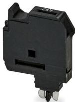
Fuse plug, Prior to replacing the cartridge fuse, disconnect the fuse connector from the basic terminal block., nom. voltage: 24 V, nominal current: 6.3 A, fuse type: G / 5 x 20, mounting type: Plug-in mounting, color: black
