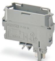
Component connector, for installing components that can be individually selected up to a diameter of 10 mm and power dissipation of up to 1 W, nom. voltage: 400 V, nominal current: 10 A, connection method: Plug-in connection, depth: 37.5 mm, width: 12.3 mm, height: 41.2 mm, number of positions: 1, color: gray, mounting type: Pluggable (slot)
