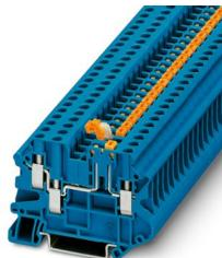
Knife-disconnect terminal block, nom. voltage: 500 V, nominal current: 20 A, connection method: Screw connection, Rated cross section: 4 mm<sup>2</sup>, cross section: 0.14 mm<sup>2</sup> - 6 mm<sup>2</sup>, mounting: NS 35/7,5, NS 35/15, color: blue
