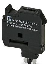
Fuse plug, Prior to replacing the cartridge fuse, disconnect the fuse connector from the basic terminal block., nom. voltage: 24 V, nominal current: 6.3 A, fuse type: G / 5 x 20, color: black
