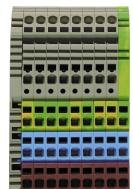
Initiator terminal / actuator terminal, Tension-spring connection, Mounting type: Mounting rail TS 35/7.5, Rated cross-section: 1.5 mm<sup>2</sup>, Width: 51 mm, Colour: Multi-coloured
