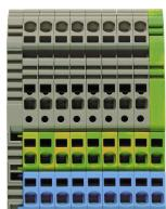
Initiator terminal / actuator terminal, Tension-spring connection, Mounting type: Mounting rail TS 35/7.5, Rated cross-section: 1.5 mm<sup>2</sup>, Width: 61.2 mm, Colour: Multi-coloured
