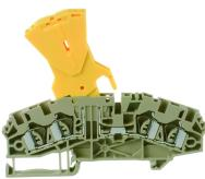
Fuse-disconnect terminal, Tension-spring connection, Mounting type: Mounting rail TS 35/7.5, Rated cross-section: 2.5 mm<sup>2</sup>, Width: 5.1 mm, Colour: Beige
