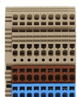
Initiator terminal / actuator terminal, Tension-spring connection, Mounting type: Mounting rail TS 35/7.5, Rated cross-section: 1.5 mm<sup>2</sup>, Width: 51 mm, Colour: Multi-coloured
