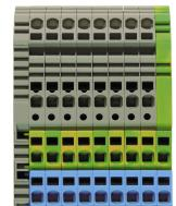
Initiator terminal / actuator terminal, Tension-spring connection, Mounting type: Mounting rail TS 35/7.5, Rated cross-section: 1.5 mm<sup>2</sup>, Width: 51 mm, Colour: Multi-coloured
