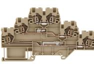
Three-level initiator terminal | Multi-wire terminal, Tension-spring connection, Mounting type: Mounting rail TS 35/7.5, Rated cross-section: 2.5 mm<sup>2</sup>, Width: 5.1 mm, Colour: Beige
