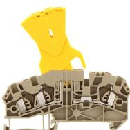
Fuse-disconnect terminal, Tension-spring connection, Mounting type: Mounting rail TS 35/7.5, Rated cross-section: 2.5 mm<sup>2</sup>, Width: 5.1 mm, Colour: Beige
