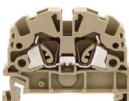
Feed-through terminal, Tension-spring connection, Mounting type: Mounting rail TS 35/7.5, Rated cross-section: 2.5 mm<sup>2</sup>, Width: 5.1 mm, Colour: Beige
