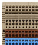
Initiator terminal / actuator terminal, Tension-spring connection, Mounting type: Mounting rail TS 35/7.5, Rated cross-section: 1.5 mm<sup>2</sup>, Width: 56.1 mm, Colour: Multi-coloured
