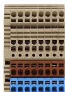
Initiator terminal / actuator terminal, Tension-spring connection, Mounting type: Mounting rail TS 35/7.5, Rated cross-section: 1.5 mm<sup>2</sup>, Width: 45.9 mm, Colour: Multi-coloured
