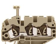
Feed-through terminal, Tension-spring connection, Mounting type: Mounting rail TS 15/5.5, Rated cross-section: 2.5 mm<sup>2</sup>, Width: 5.1 mm, Colour: Beige
