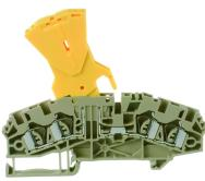
Fuse-disconnect terminal, Tension-spring connection, Mounting type: Mounting rail TS 35/7.5, Rated cross-section: 2.5 mm<sup>2</sup>, Width: 5.1 mm, Colour: Beige
