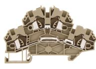
Double-level terminal, Tension-spring connection, Mounting type: Mounting rail TS 35/7.5, Rated cross-section: 2.5 mm<sup>2</sup>, Width: 5.1 mm, Colour: Beige
