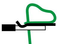
Feed-through terminal, Tension-spring connection, Mounting type: Plug in, Rated cross-section: 2.5 mm<sup>2</sup>, Width: 66.3 mm, Colour: Beige
