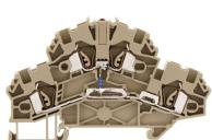
Double-level terminal with electronic components, Tension-spring connection, Mounting type: Mounting rail TS 35/7.5, Rated cross-section: 2.5 mm<sup>2</sup>, Width: 5.1 mm, Colour: Beige
