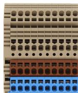
Initiator terminal / actuator terminal, Tension-spring connection, Mounting type: Mounting rail TS 35/7.5, Rated cross-section: 1.5 mm<sup>2</sup>, Width: 56.1 mm, Colour: Multi-coloured
