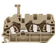
Ex feed-through terminal ATEX-certified, Tension-spring connection, Mounting type: Mounting rail TS 35/7.5, Rated cross-section: 2.5 mm<sup>2</sup>, Width: 5.1 mm, Colour: Beige
