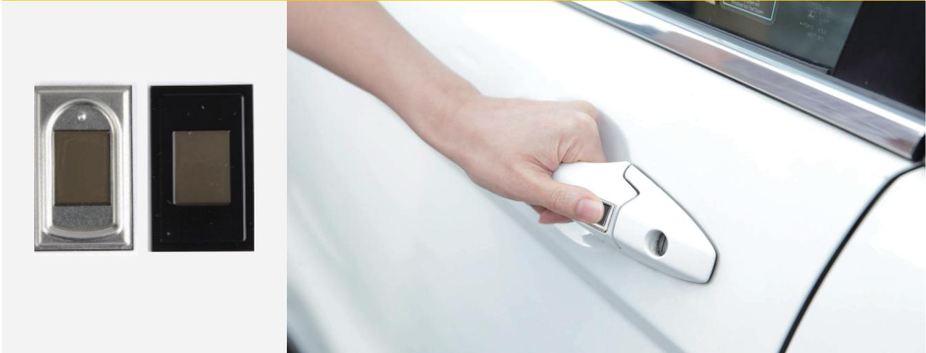
Embed the MFC-1208 compact capacitive-contact fingerprint image sensor in your product for advanced fingerprint acquisition and verification. 508 DPI resolutions delivers superior image quality for highly accurate readings and a 0.07 second read out time enable quick verification.
