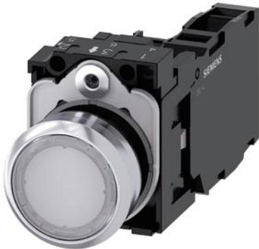
Illuminated pushbutton, 22 mm, round, metal, shiny, white, pushbutton, flat, momentary contact type, with holder, 1 NO+1 NC, LED module with integrated LED 24 V AC/DC, screw terminal, with laser labeling, lower case
