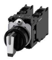
Selector switch, illuminable, 22 mm, round, plastic, white, selector switch, short, 3 switch positions I-O-II, latching, 10:30h/12h/13:30h, with holder, 2 x 1 NO+1 NC, spring-type terminal, with laser labeling, lower case
