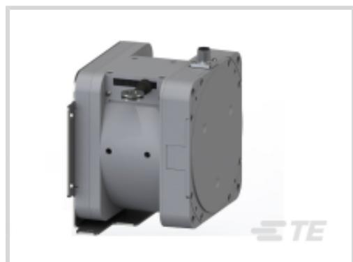
Position Sensor Product Type: **SK Series, IP67 String Pots**Full Stroke Range: **10160 mm [ 400 in ]**Output Signal Type: **CAN J1939**Accuracy: **±.35 % of FS**Repeatability: **.02 % of FS**[All IP67 String Potentiometer CANJ1939 \(2\)](#)
