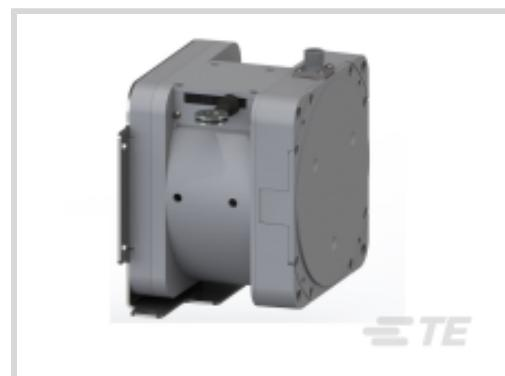
Position Sensor Product Type: **SK Series, IP67 String Pots**Full Stroke Range: **10160 mm [ 400 in ]**Output Signal Type: **0 - 10 VDC, 4 - 20 mA**Accuracy: **±.35 % of FS**Repeatability: **.02 % of FS**[All IP67 String Potentiometer, 0-10V / 4-20MA \(2\)](#)
