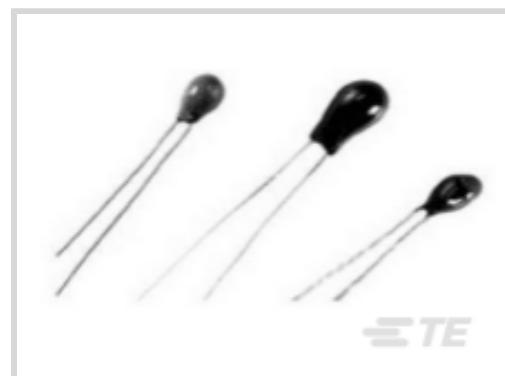
NTC Sensor Type: **Epoxy Coated NTC Thermistor**Lead Wire Length: **76 mm [ 2.992 in ]**Resistance (at 25°C): **30 kΩ** $\beta$ -Value(25/85): **3943 K**Tolerance  $\beta$ -Value:  **$\pm 0.4 \%$** [All Model 44000 Series \(32\)](#)
