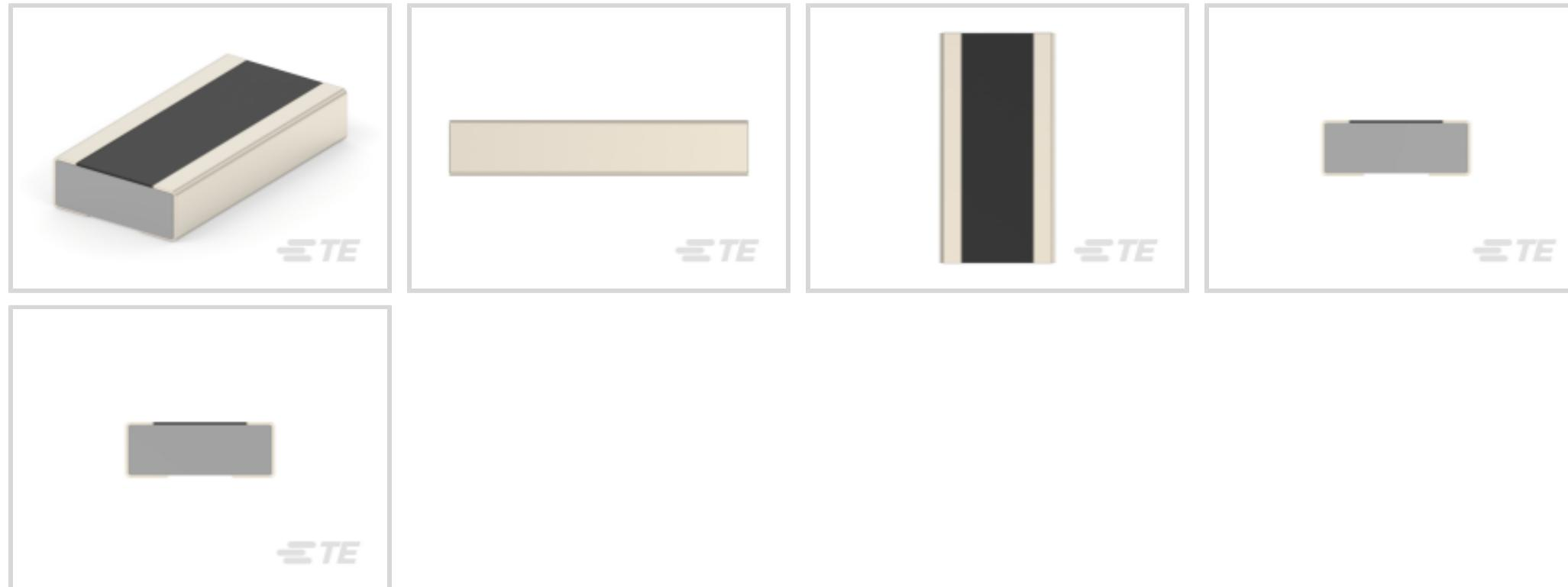
Resistor Type: **Current Sensing Resistor**Element Type: **Thick Film**Package Size Code: **0612**Power Rating: **.75 W**Resistance Value: **.027  $\Omega$**
