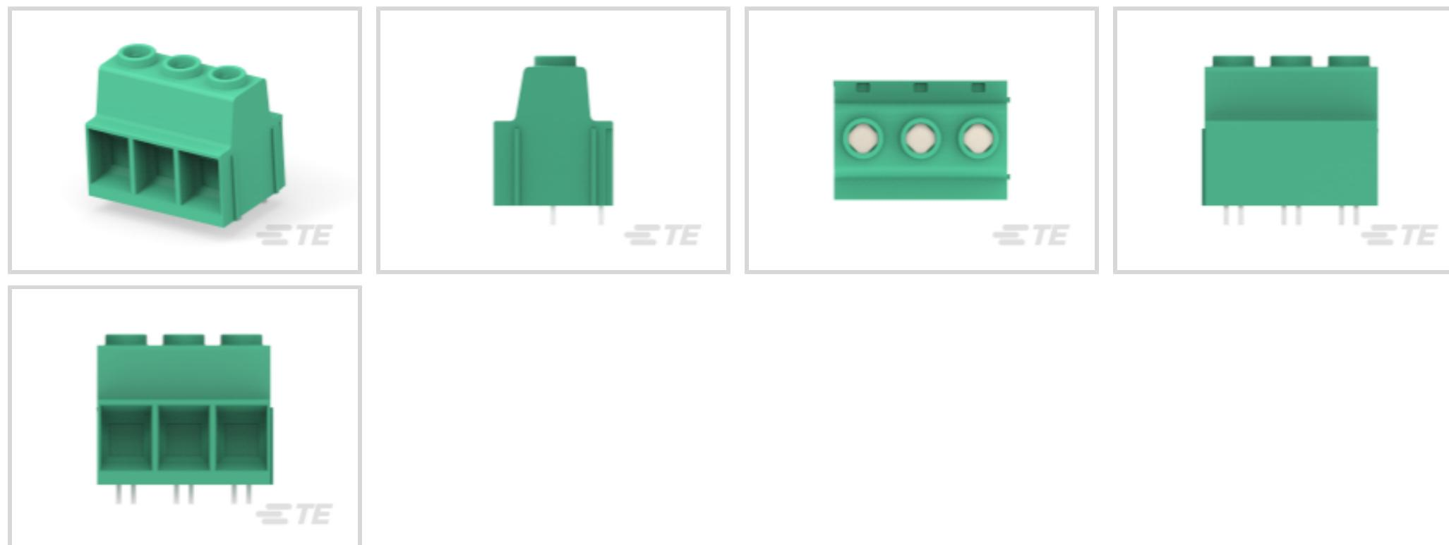
Terminal Block Connector Type: **Header**Connector System: **Wire-to-Component**Number of Positions: **3**Centerline (Pitch): **15 mm [.591 in]**Number of Rows: **2**
