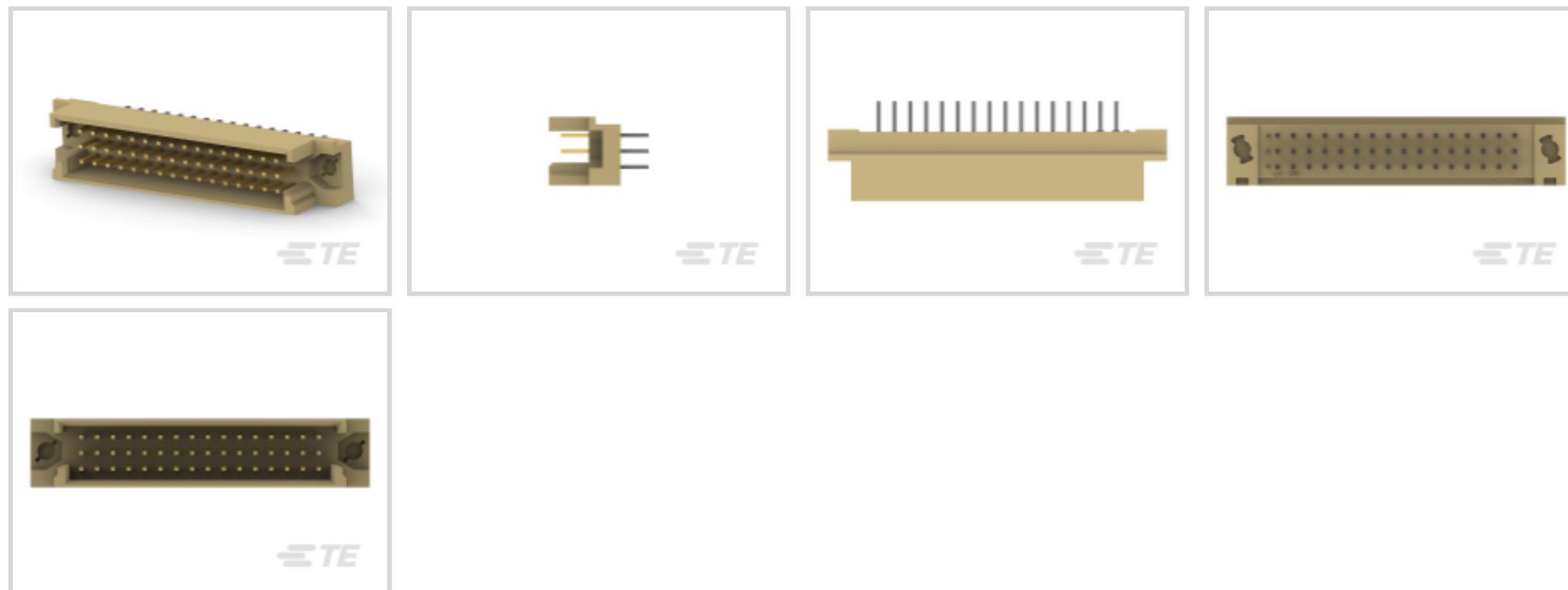
Connector & Housing Type: **Plug**Connector System: **Board-to-Board**Termination Post & Tail Length: **4.5 mm [ .177 in ]**Number of Positions: **48**Centerline (Pitch): **2.54 mm [ .1 in ]**
