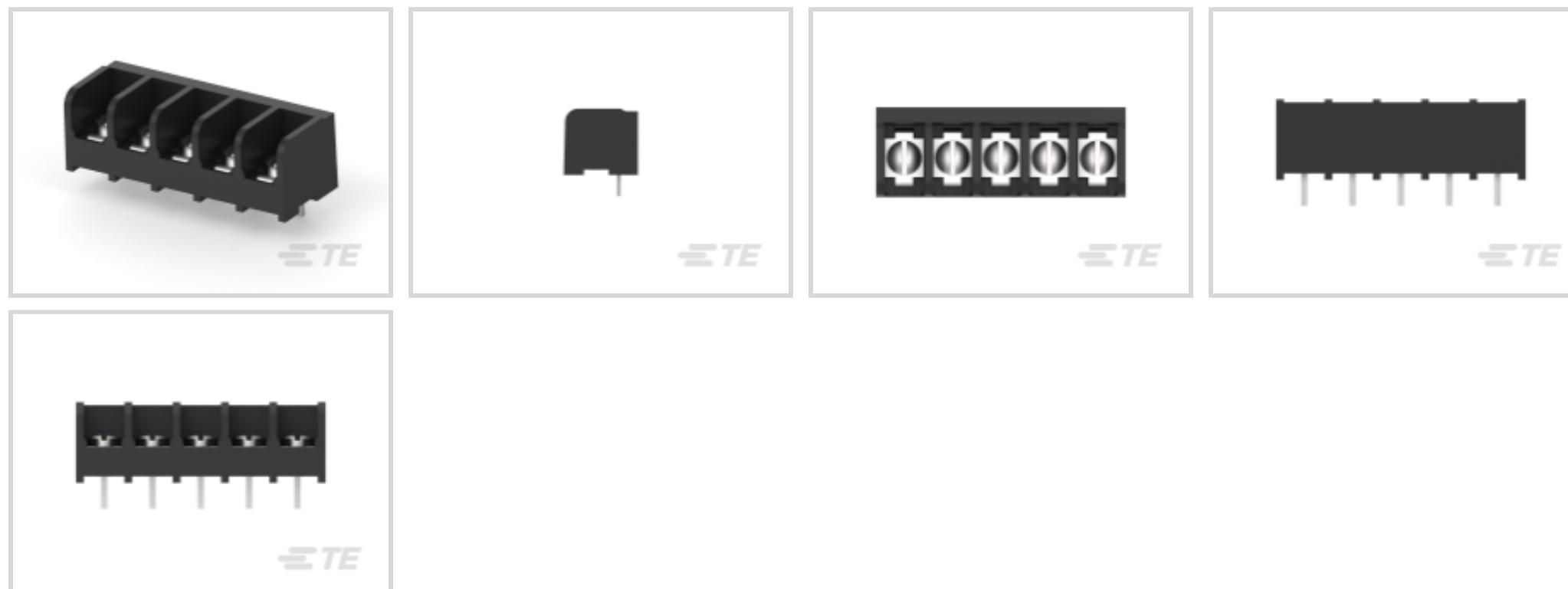
Barrier Strip Style: **Tri-Barrier**Bottom Termination Type: **Printed Circuit Pin**Connector System: **Wire-to-Board**Number of Positions: **5**Centerline (Pitch): **9.53 mm [.375 in]**
