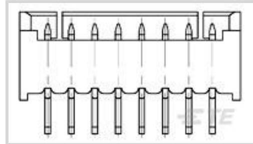
Connector System: **Wire-to-Board**Number of Positions: **15**Number of Rows: **1**Centerline (Pitch): **1.25 mm [.049 in]**PCB Mount Orientation: **Vertical**[All AMP HPI 1.25 mm Headers \(0\)](#)
