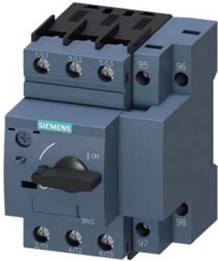
Circuit breaker size S0 for motor protection, CLASS 10 with overload relay function A-release 10...16 A N-release 208 A screw terminal Standard switching capacity
