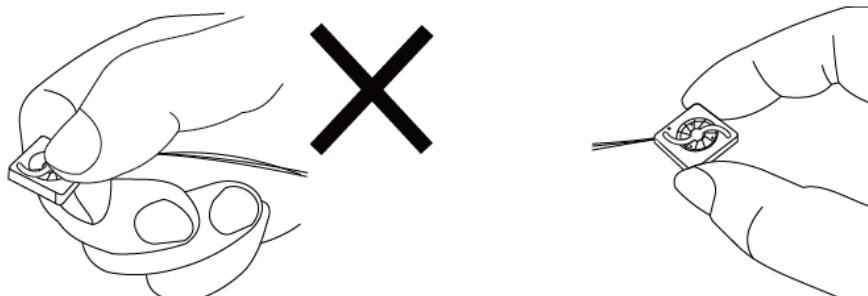
**Don't pull fan with lead wires.**
