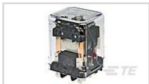
Relay Type: **Industrial Panel Plug-In**Coil Magnetic System: **Monostable, AC**Coil Power Rating Class: **[ 2 - 3 VA ]**Coil Power Rating AC: **2 VA**Coil Resistance: **2250 Ω**
