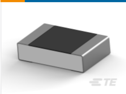
TE Part # 3-2176380-3 RQ 0805 2K49 0.1% 10PPM 5K RL
