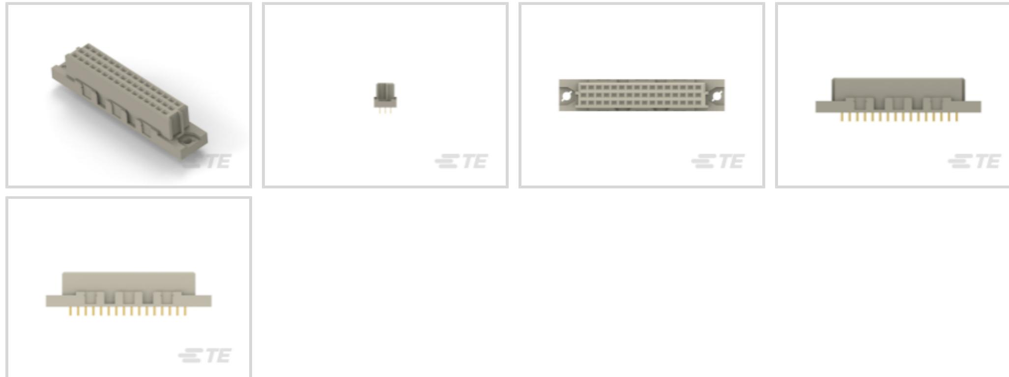
Connector & Housing Type: **Receptacle**Connector System: **Board-to-Board**Termination Post & Tail Length: **2.9 mm [.114 in]**Number of Positions: **48**Centerline (Pitch): **2.54 mm [.1 in]**
