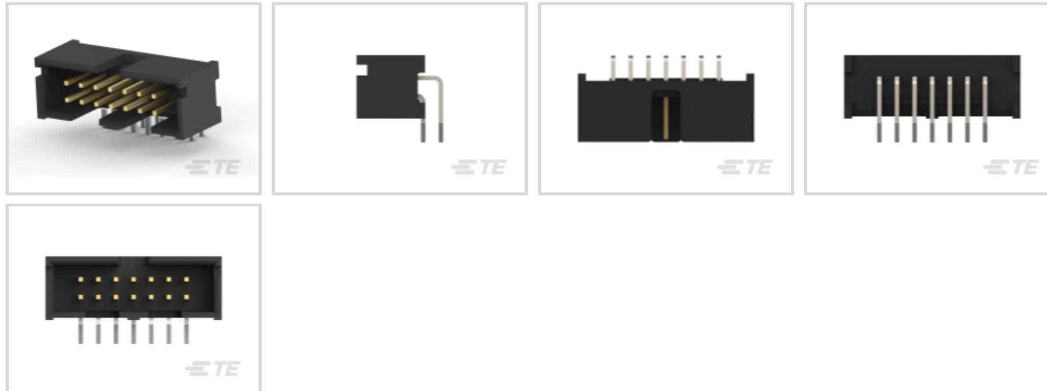
Connector System: **Board-to-Board**Number of Positions: **14**Centerline (Pitch): **2.54 mm [.1 in]**PCB Mount Retention: **Without**PCB Mount Orientation: **Right Angle**
