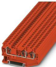
Feed-through terminal block, nom. voltage: 800 V, nominal current: 32 A, number of connections: 3, connection method: Spring-cage connection, 1 level, Rated cross section: 4 mm<sup>2</sup>, cross section: 0.08 mm<sup>2</sup> - 6 mm<sup>2</sup>, mounting type: NS 35/7,5, NS 35/15, color: red
