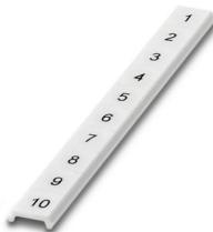
Zack Marker strip, flat, Strip, white, labeled, Printed vertically: consecutive numbers 1 ... 10, 11 ... 20, etc. up to 91 ... 100, mounting type: snapped, for terminal block width: 6.2 mm, lettering field size: 5.15 x 6.15 mm, Number of individual labels: 10
