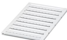
Marker for terminal blocks, Sheet, white, unlabeled, can be labeled with: BLUEMARK ID COLOR, BLUEMARK ID, BLUEMARK CLED, PLOTMARK, CMS-P1-PLOTTER, mounting type: snapped, for terminal block width: 6.2 mm, lettering field size: 5.6 x 5.1 mm, Number of individual labels: 80
