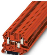
Feed-through terminal block, nom. voltage: 500 V, nominal current: 32 A, number of connections: 3, connection method: Screw connection, Rated cross section: 4 mm<sup>2</sup>, cross section: 0.14 mm<sup>2</sup> - 6 mm<sup>2</sup>, mounting type: NS 35/7,5, NS 35/15, color: red
