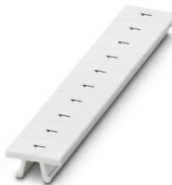
Zack marker strip, Strip, white, labeled, can be labeled with: CMS-P1-PLOTTER, printed horizontally: Identical numbers 1 or 2, etc. up to 100, mounting type: snapped, for terminal block width: 6.2 mm, lettering field size: 6.15 x 10.5 mm, Number of individual labels: 10
