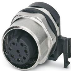
Device connector front mounting, 8-position, Socket, angled, M12-SPEEDCON, coding: A, Front mounting, M12 x 1, Solder pins, Alternative product in accordance with RoHS II without Exemption 6c (Pb < 0.1 %) item no.: 1239643
