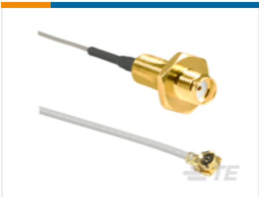
TE Part # CSI-SGFE-100-UFFR SMA to U.FL/MHF1 100mm 1.13 OD
